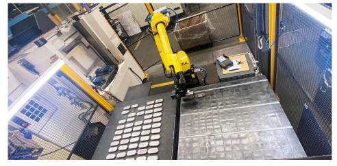
the system's ability to detect and handle stacks of random parts with precision. This rigorous testing phase included imaging and programming paths for a variety of components, ensuring the system could seamlessly adapt to production demands.
